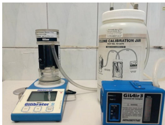
Fig. 3. A set for checking the flow of air in the aspirator together with the aspirator type GilAir3 (photo K. Pikulik)
