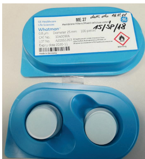
Fig. 2. An example of a membrane filter of cellulose esters of the diameter \varnothing 25 mm intended for testing the inhaled fraction (photo K. Pikulik)
