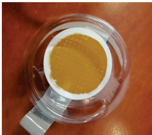
Fig. 1. An example of a filter of the diameter Ø37 mm intended for testing the respirable fraction (photo K. Pikulik)
