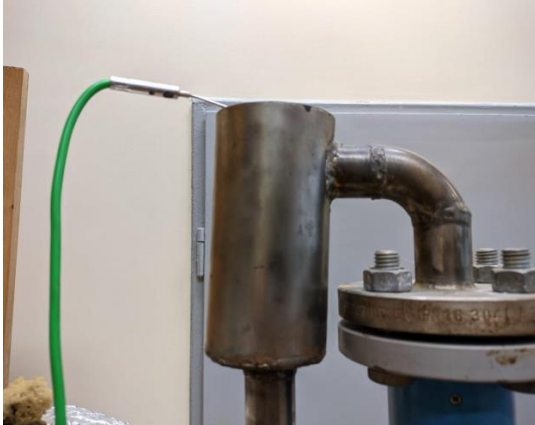
Fig. 2. a) The first thermocouple probe of the DO9416 thermometer located at the inlet of the calorimeter in the overflow vessel, measuring the T_1 temperature; b) the second thermocouple probe of the DO9416 thermometer located at the outlet of the calorimeter, measures the T_2 temperature (own study)
