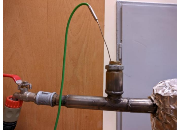
Fig. 2. a) The first thermocouple probe of the DO9416 thermometer located at the inlet of the calorimeter in the overflow vessel, measuring the T_1 temperature; b) the second thermocouple probe of the DO9416 thermometer located at the outlet of the calorimeter, measures the T_2 temperature (own study)
